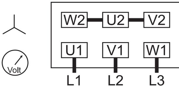
Double star connection, multi-voltage motor (low voltage):
