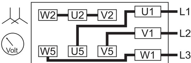
Star connection, multi-voltage motor (high voltage):
