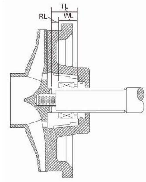
*Figure E-1: FMI Seal Chamber*
