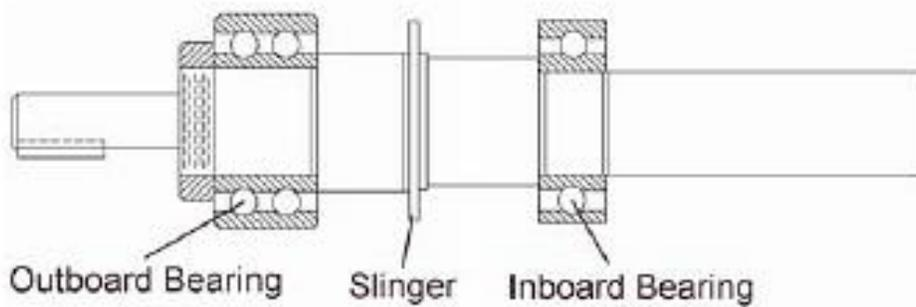
Figure V-1: Typical Shaft Arrangement
