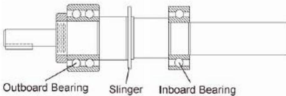
Figure V-1: Typical Shaft Arrangement
