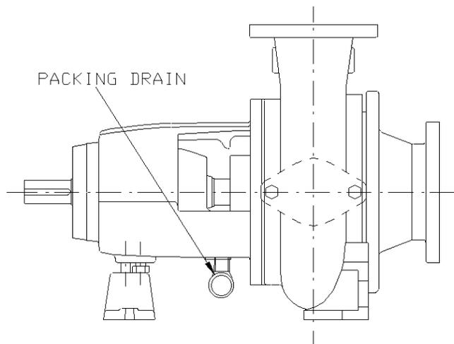
Figure I-6: Packing Drain
