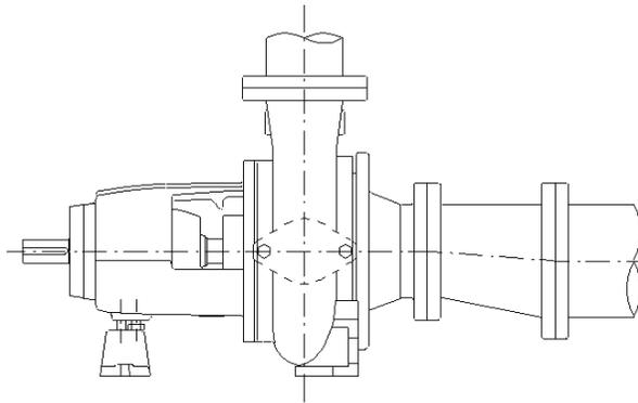
Figure I-3: Recommended Suction Piping
