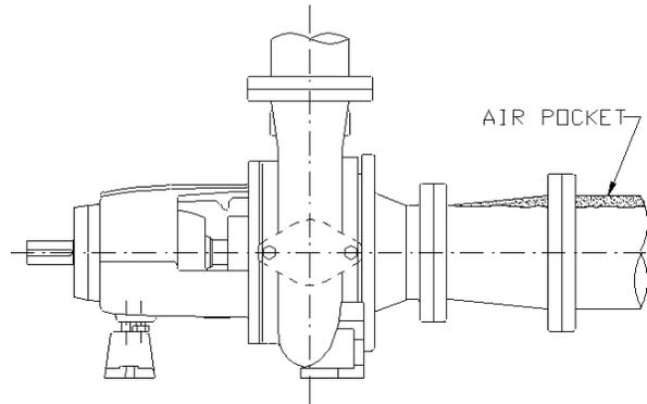
Figure I-4: Incorrect Suction Piping
