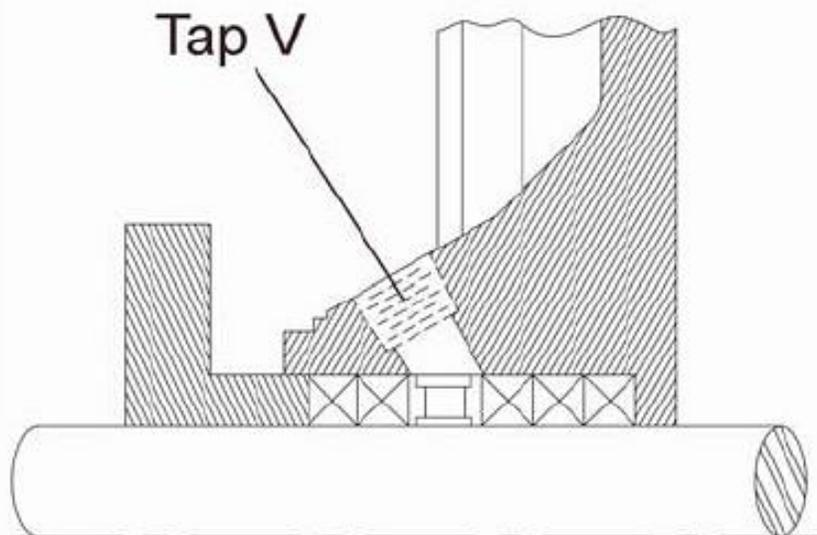
*Figure I-5: Packing Flush Connection*
